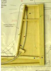
19. Install Elevator control cable in
